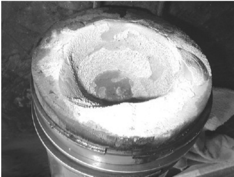
Figure 1: Silicon oxide deposits on a gas engine piston.
